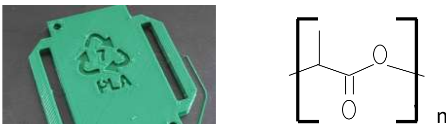
Figure 2: (a) Plastic sheet form of PLA (b) PLA chemical formula [15]
