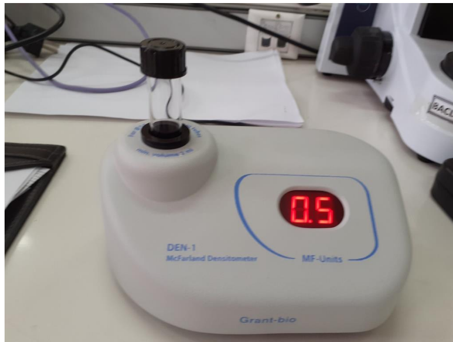
McFarland Densitometer used for checking turbidity during antimicrobial testing
