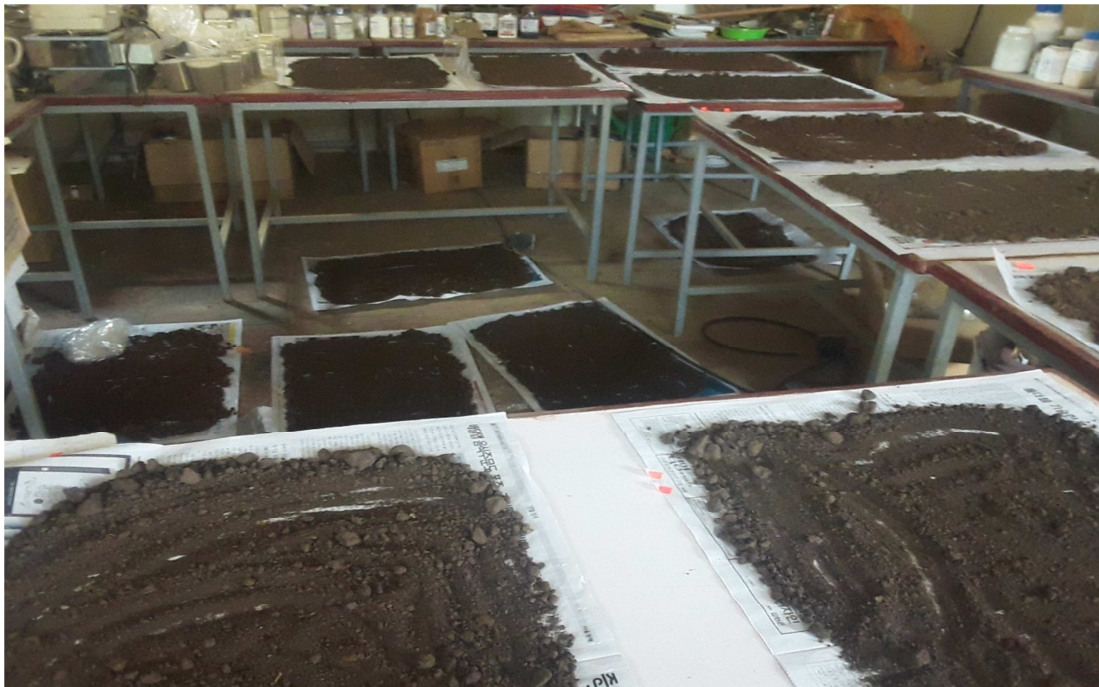
Air Drying of the Soil Samples Under Shade on Spread Sheet (Picture by the Author)
