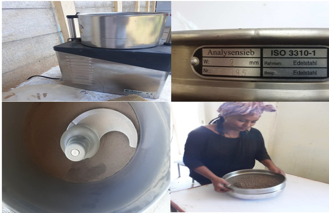
Grinding and sieving the air dried soil samples for further soil physicochemical analysis (Picture by the Author)
