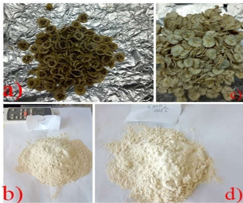
Figure 3.3: SMBS & Hot water pretreated banana slice and flour . a) hot water pretreated banana slices, b) hot water pretreated banana flour, c) SMBS pretreated banana slices and d) SMBS pretreated banana flour
