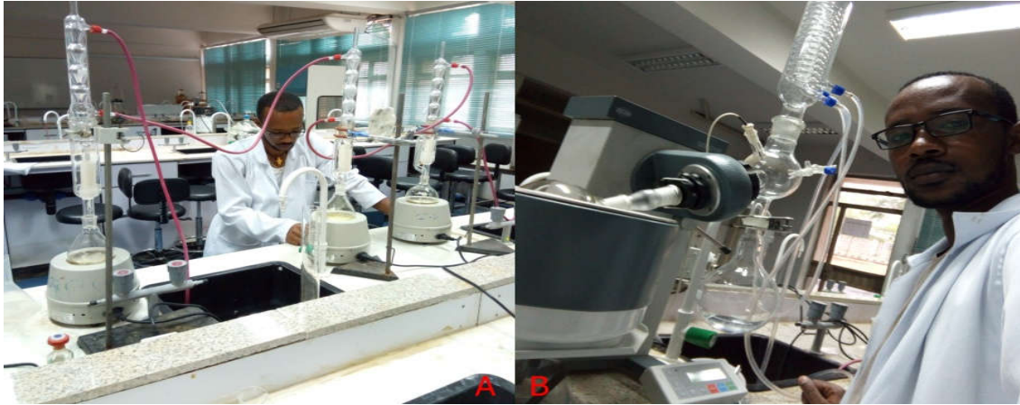
Figure 3.4: Crude fat laboratory extraction a) Soxhlet-extraction and b) Rotary evaporator
