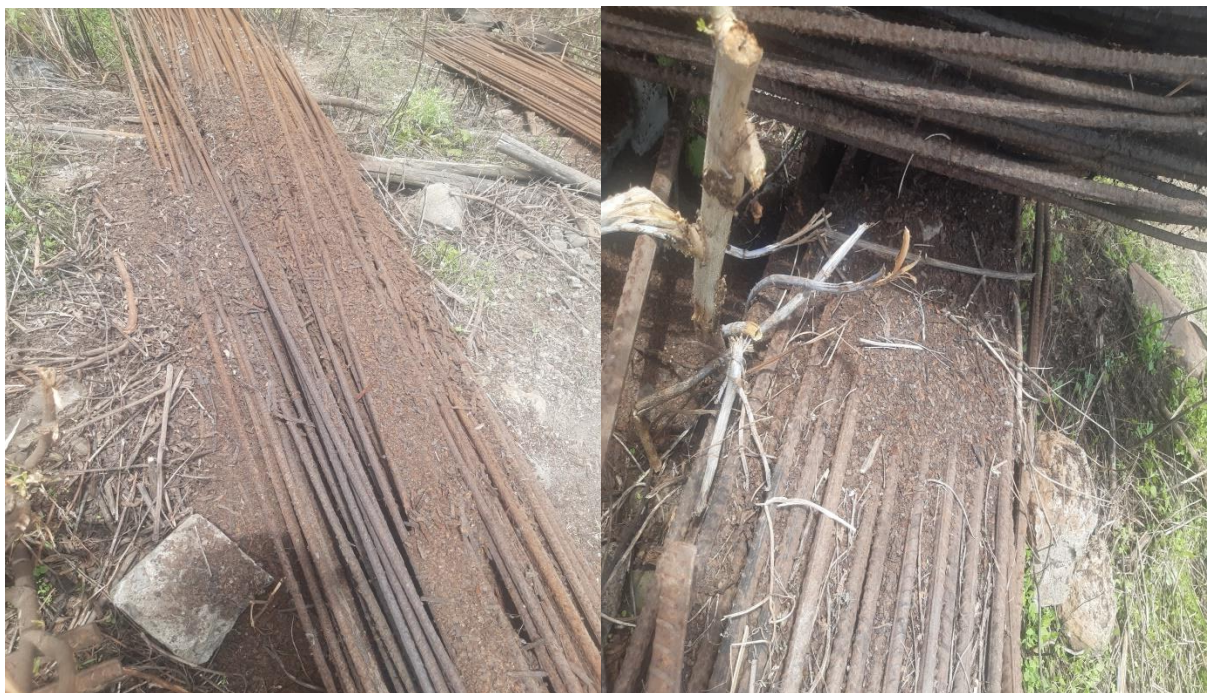
Rebar stored for long period of time
