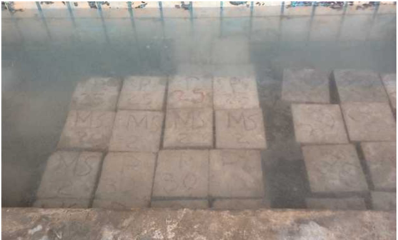
F-2 Curing specimens for reference and special C-25 and C-30 concrete mixes
