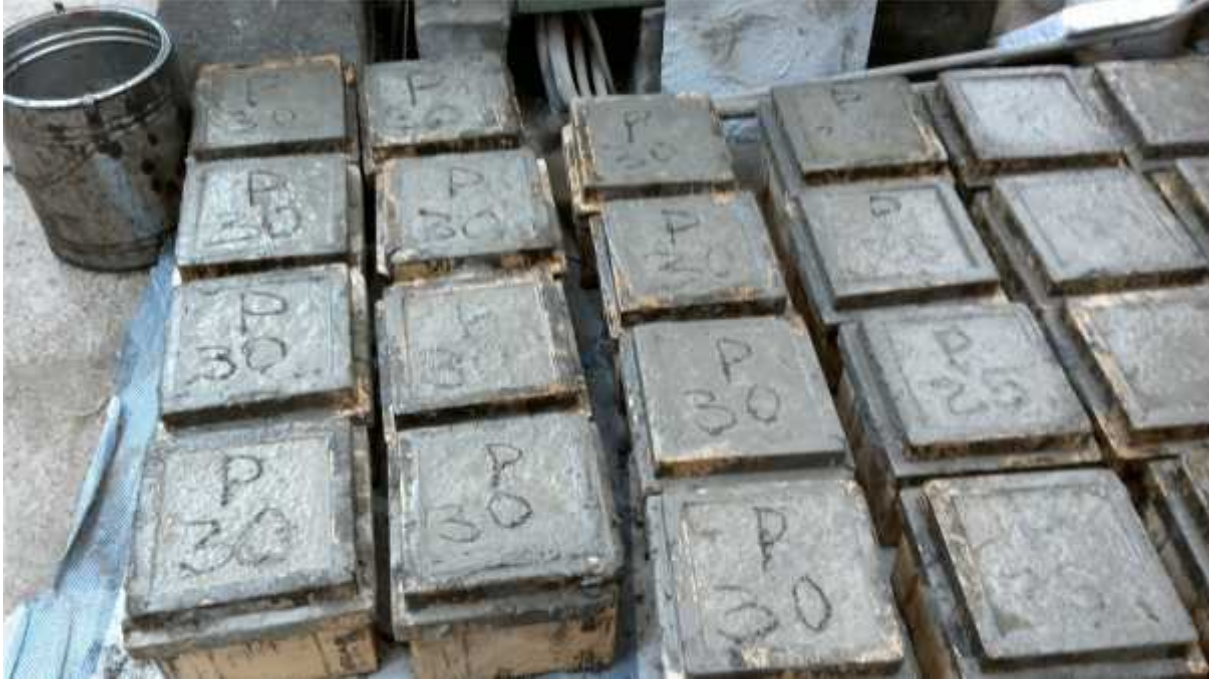
F-2 Curing specimens for reference and special C-25 and C-30 concrete mixes
