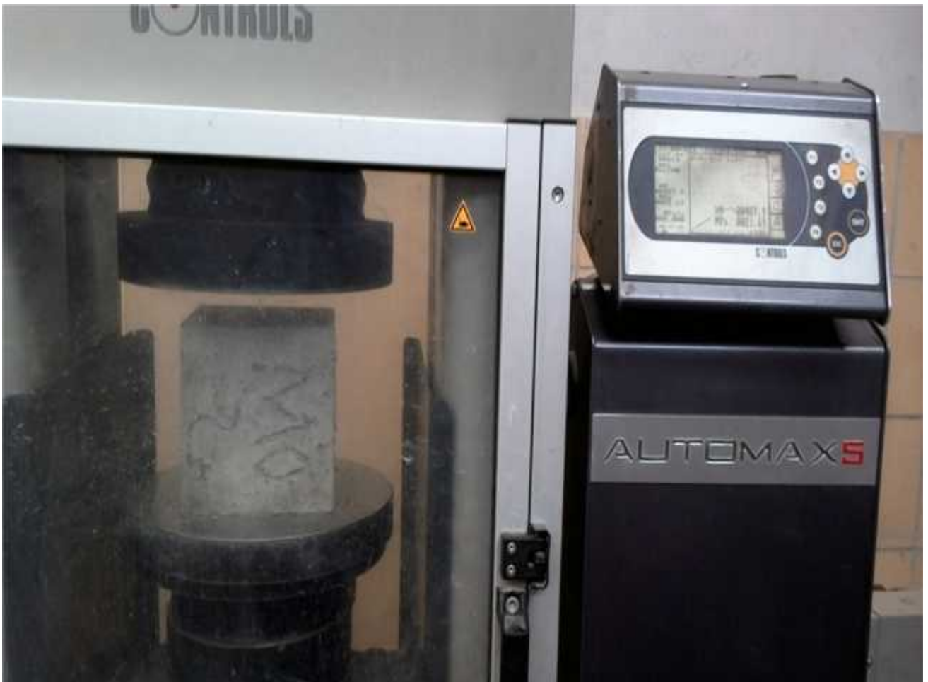
F-4 Sample concrete of C-25 (OPC), compressive strength test at 7 days
