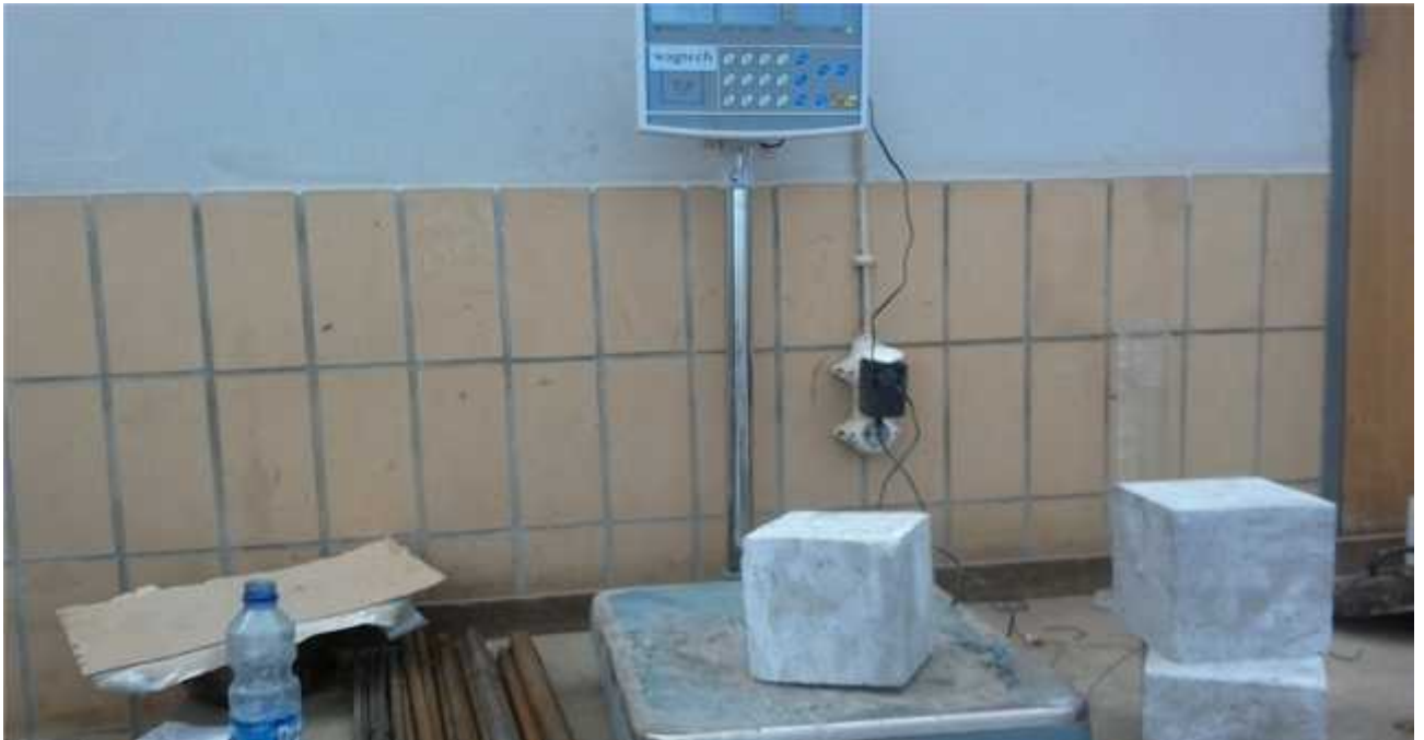
F-4 Sample concrete of C-25 (OPC), compressive strength test at 7 days
