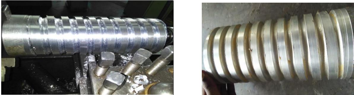
Figure 3.8: Preparing of spring mold from solid aluminum
