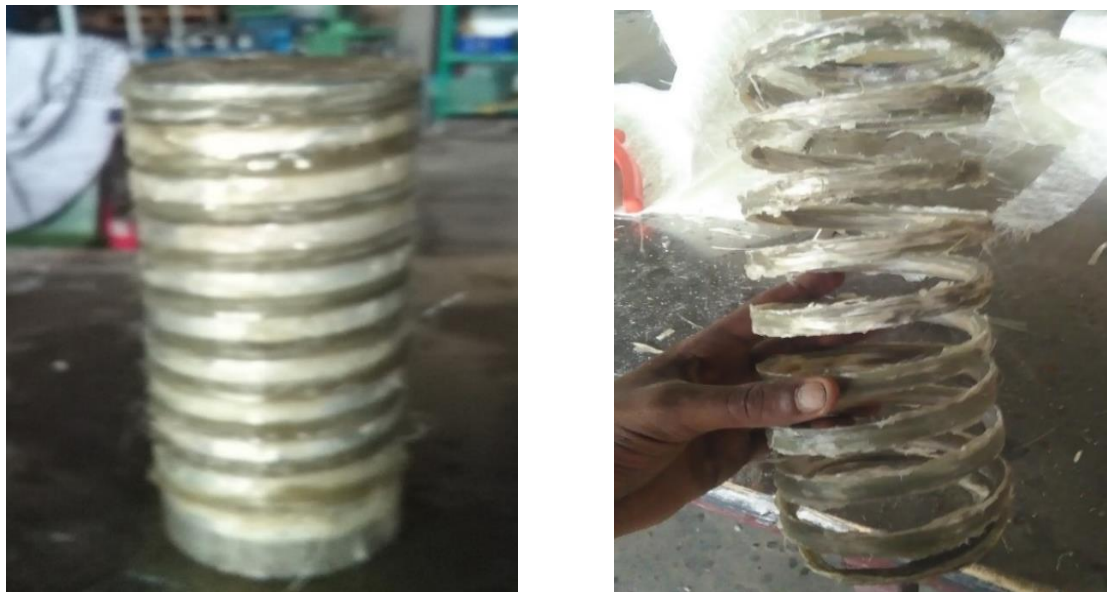
Figure 3.11: Final manufacturing of HCS made of composite material
