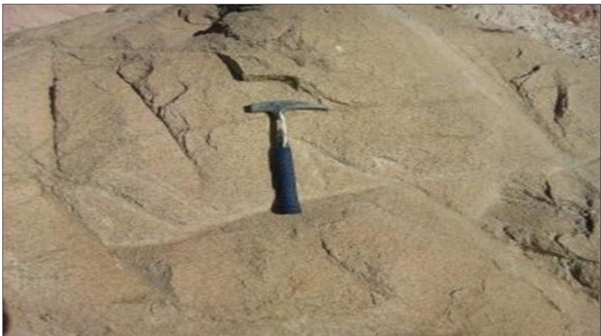
Figure 3.3: Field photo of granite having gray color and granular texture characteristics sampled at the base of the open pit.
