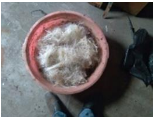
Figure 4-3 : Step-1 Dry mixing of the soil and sisal fiber
