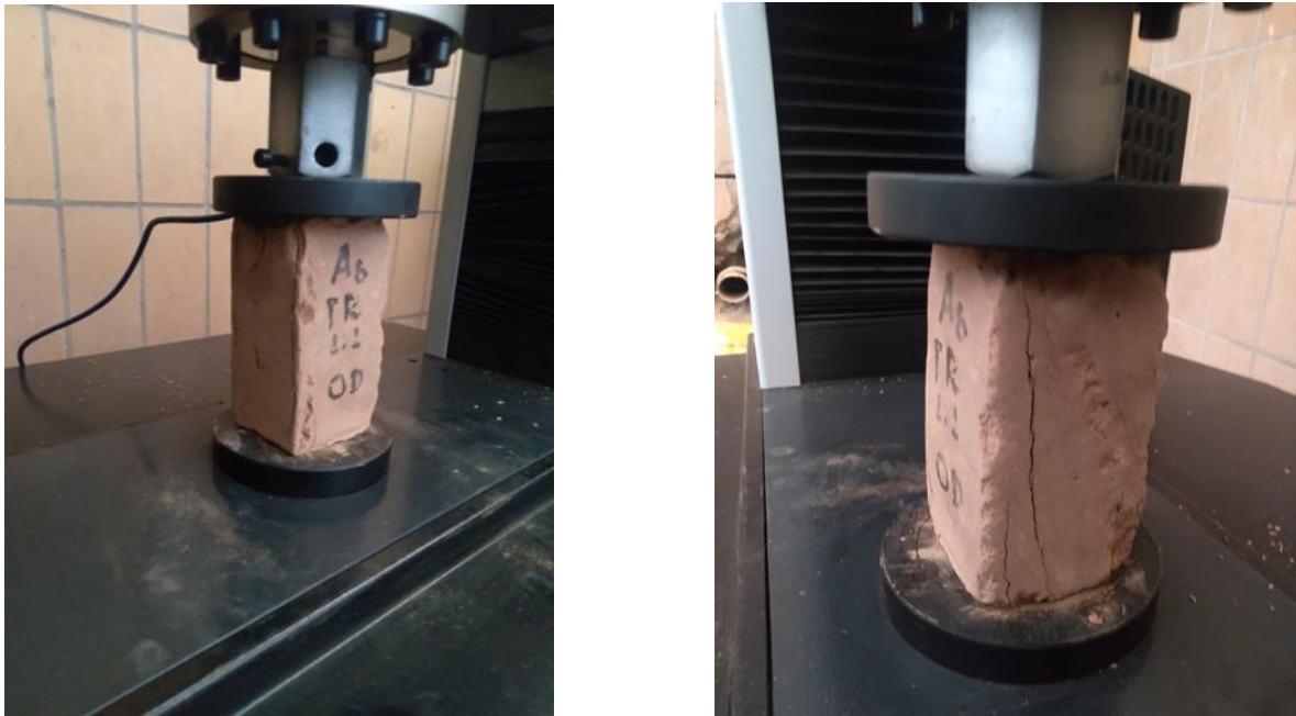
Figure 5-4 : Sample and Uniaxial testing Setup.
