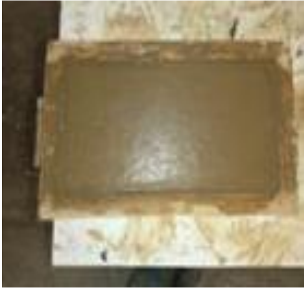
Figure 4-7 : Step-5 Smoothing bottom and top surface of the brick and gradually removing from the mould.
