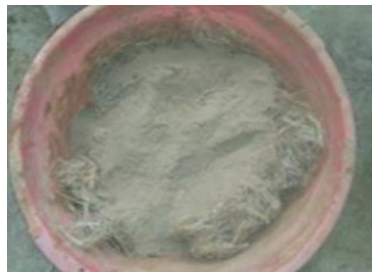
Figure 4-3 : Step-1 Dry mixing of the soil and sisal fiber
