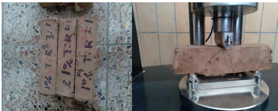
Figure 5-5 : Sample and Three point bending test setup
