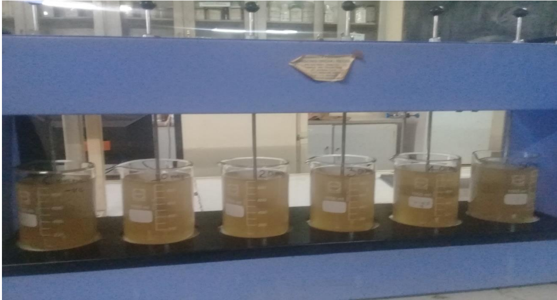
Figure 7: The image of Jar test (captured by PI at the laboratory)
