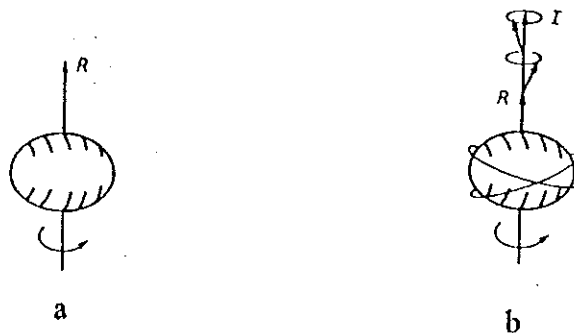
Fig. I. Two different modes of rotation generating angular momentum. (a) Collective rotation of a prolate nucleus, (b) particle alignment in an oblate nucleus.
