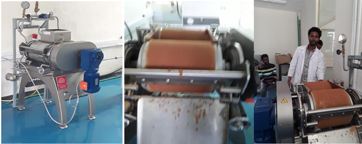
Figure anchote based instant baby food preparation using drum dryer at Addis Ababa Science and Technology University.
