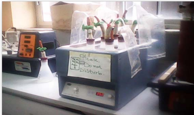
Figure3.1 Experimental set-up; shaking water bath loaded with anaerobic digesters
