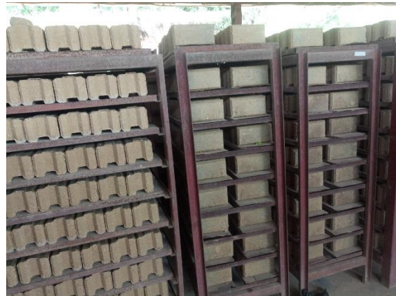
Figure 4. 18: Method of construction and storage of hydraform
