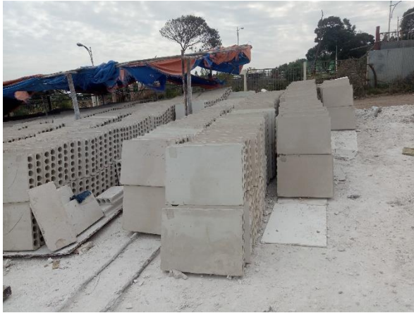
Figure 4. 14: Gypsum block at manufacturing
