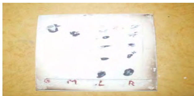
Fig 3 Spots developed from starch hydrolysates on TLC by the action of Bacillus CRC and Bacillus CLC alpha amylase
