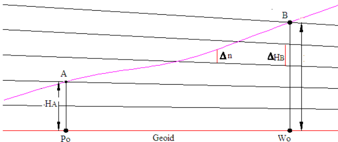
Figure 2.2: The principles of leveling and equipotential surface (Hofmann Wellenhof and Helmut Mortiz, 2005), P_o is a point on the geoid defined by a unique potential W_o .
