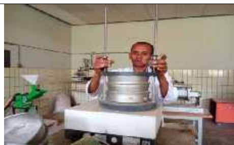
Plate 2 Sieve separation of grinded coffee husk of x size where 1mm < x < 2mm.
