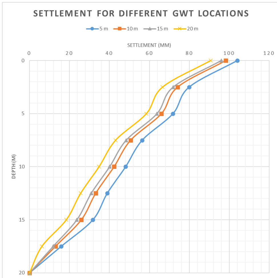
Figure 31 Settlement for different GWT locations
