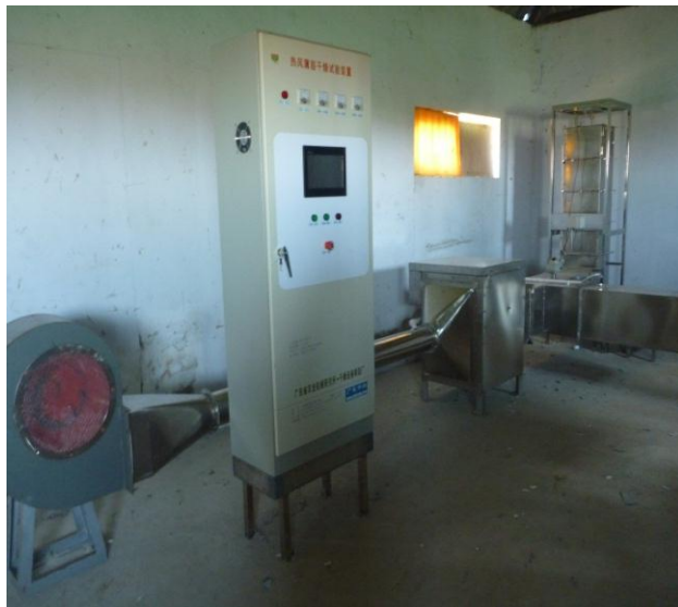
Hot thin layer dryer (GD-100, China,2016)
