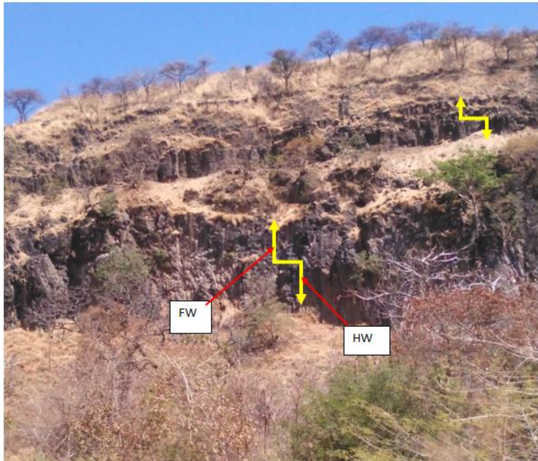
Figure 3.5: Photo illustrate normal fault, which affect the basaltic unit. HF = Hanging wall, FW = Foot Wall.
