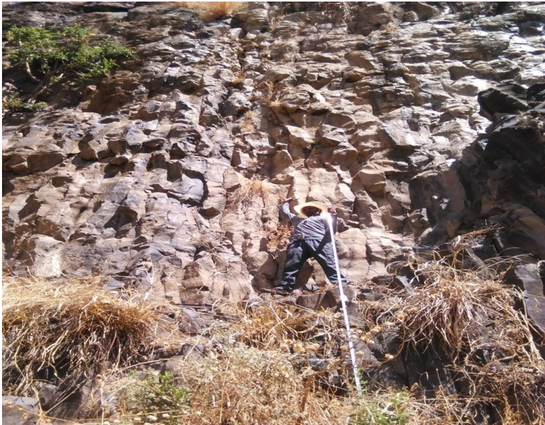
Figure: 3.3: Closely taken photo of columnar jointed basalt cropped out at northern of Ghibe Genet forestry and agricultural PLC head office to Serete Village.
