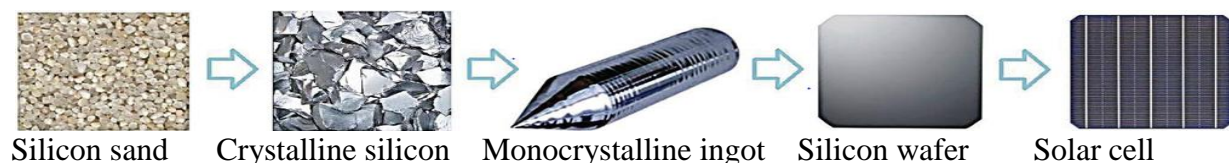
Fig.2.3. Manufacturing process of a solar cell
