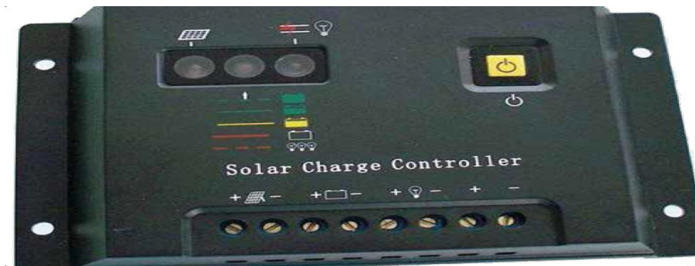
Fig.2.16 Solar battery charge controller (Solar and Development 2015)
