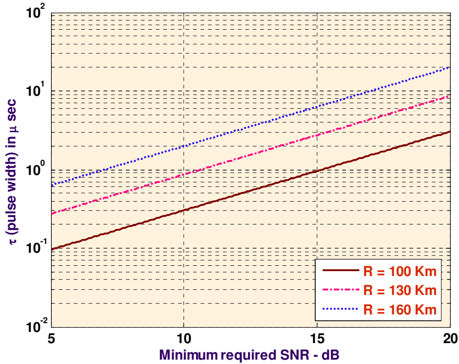
Figure 4.2 Pulse widths versus required SNR for three different detection range values.
