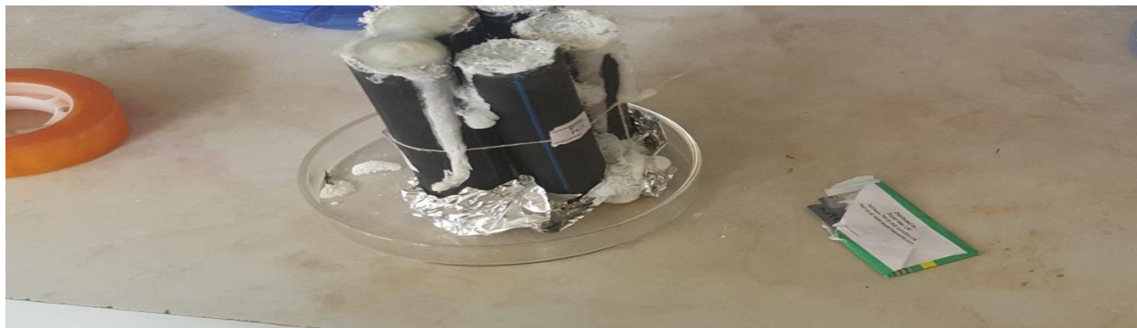
Figure 3-3 Prepared NaCl salt bridge
