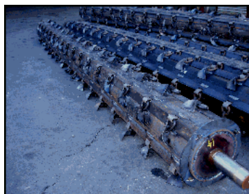
Figure 4.15: Alternative C- Knife like blades shown on the blade drum of a flail mower
