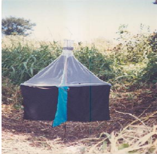
Plate 1. A mono-pyramidal trap fixed in site to capture the vector fly.
