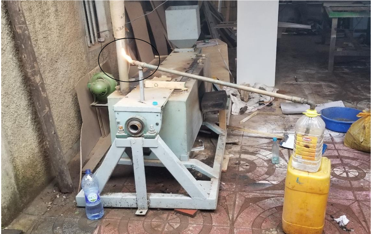
Figure 5-2 Gas production indication on first run
