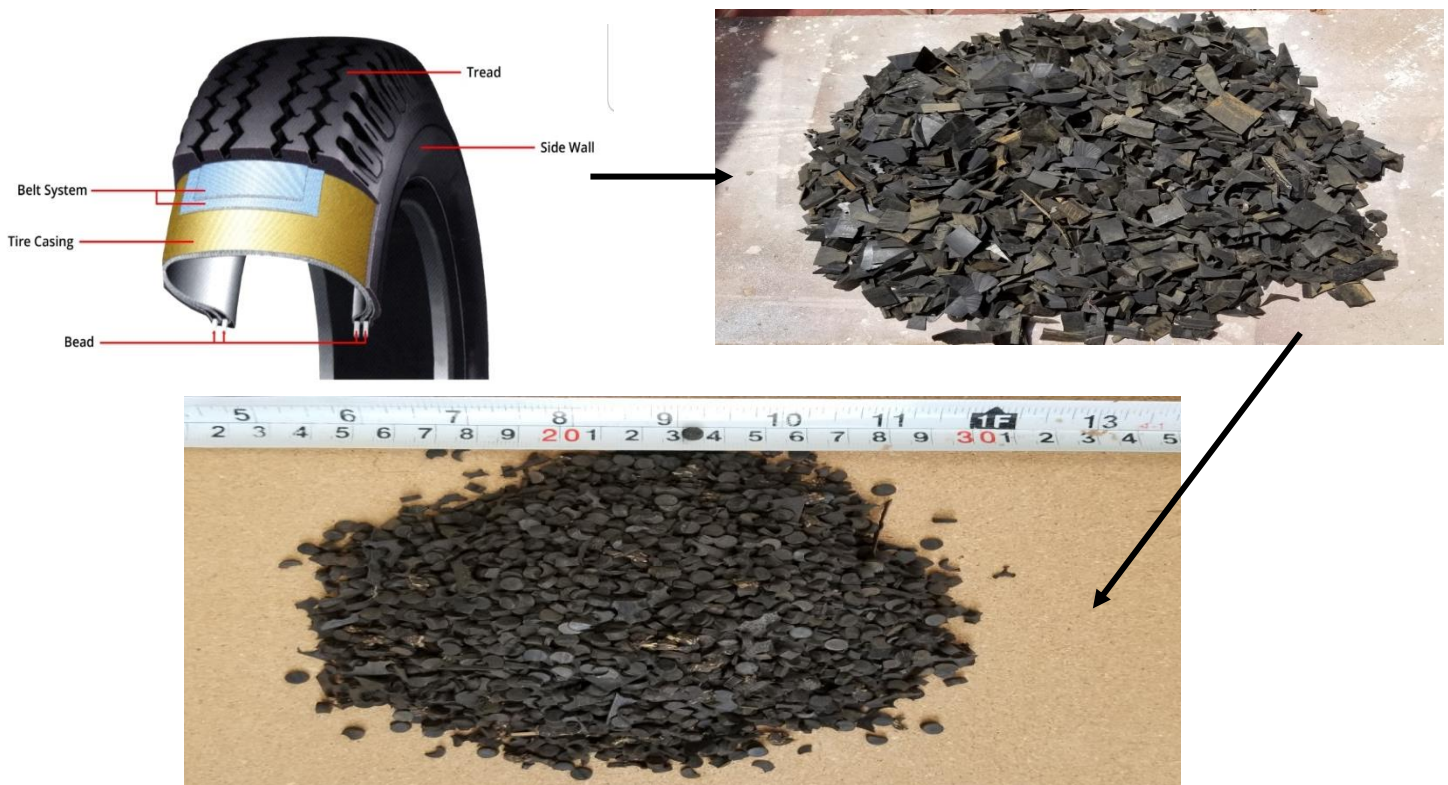
Figure 3-1 Sample tire particles ground to a size of 5 mm
