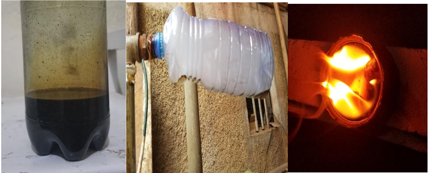
Figure 6-5 Pyro-oil/Scrap tire oil, Gas fractions with visible oil condensates and flammability test of pyro oil (left to right)
