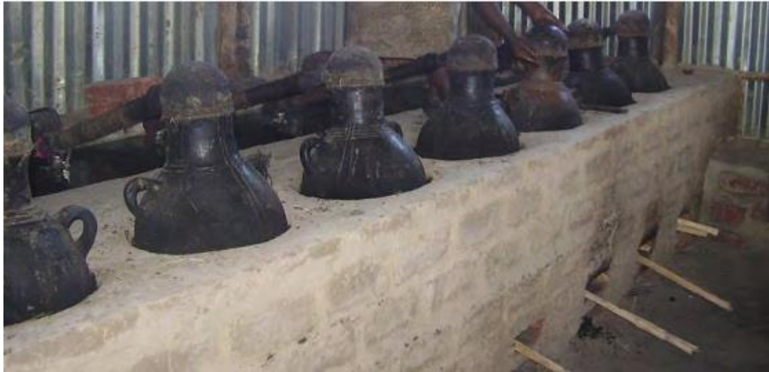
Figure 1: Biomass Areke distillation stove, (Gezahegne, 2008)
