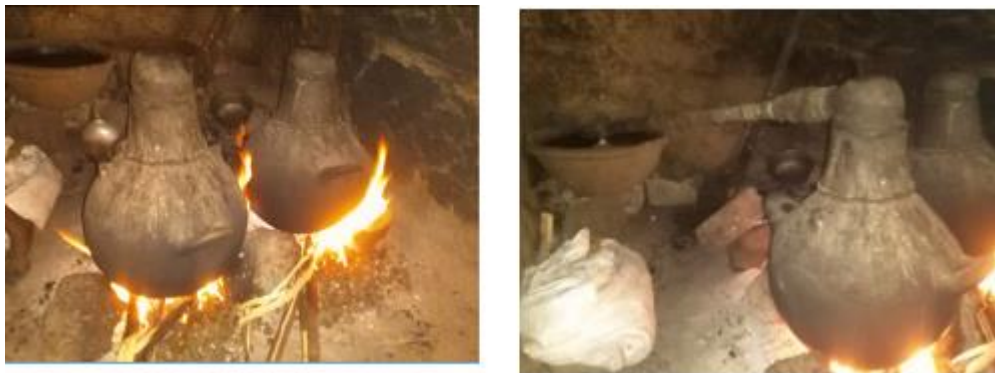
Figure 9: a) Areke difedif undergoing pre-heating process before sealed, b) Process of traditional Areke distillation
