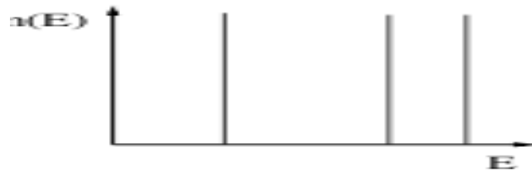
Figure 2.4: The Density of state of quantum dot (0D).
