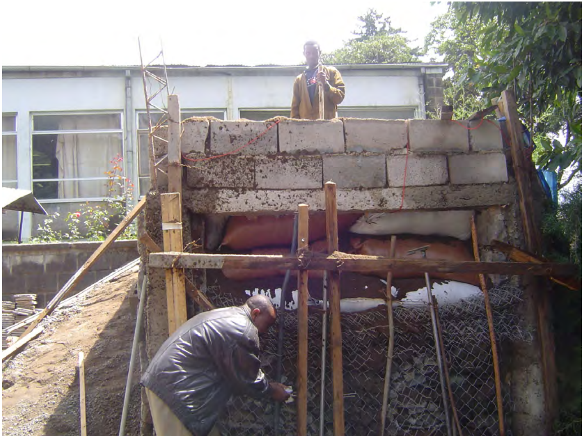
Figure C-2: The First model retaining wall, measuring the horizontal displacement of reinforcement steel by dial gauge
