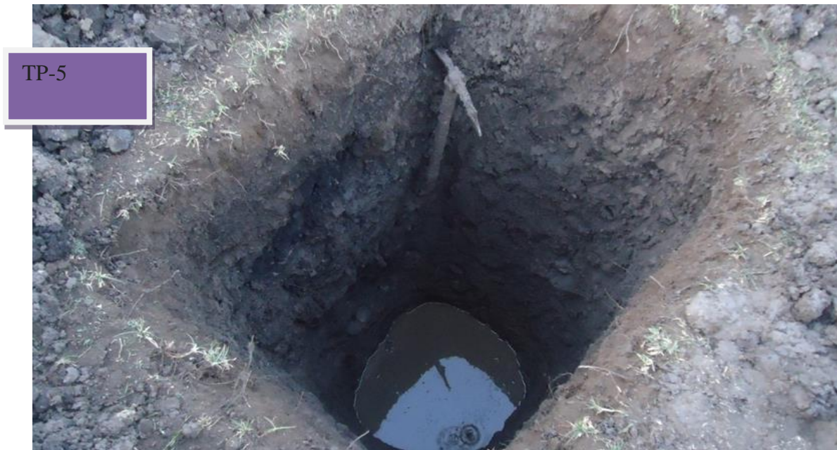
Plate.4.2 The ground water at test pit 5
