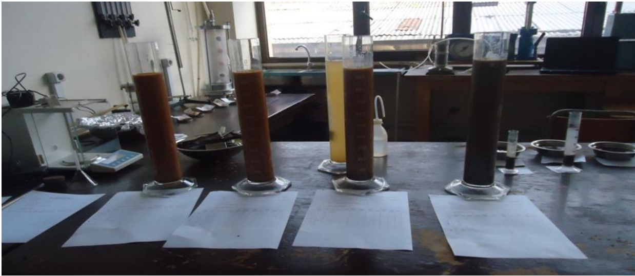
Fig.5.3 Hydrometer Analysis for fine grained soils of the study area
