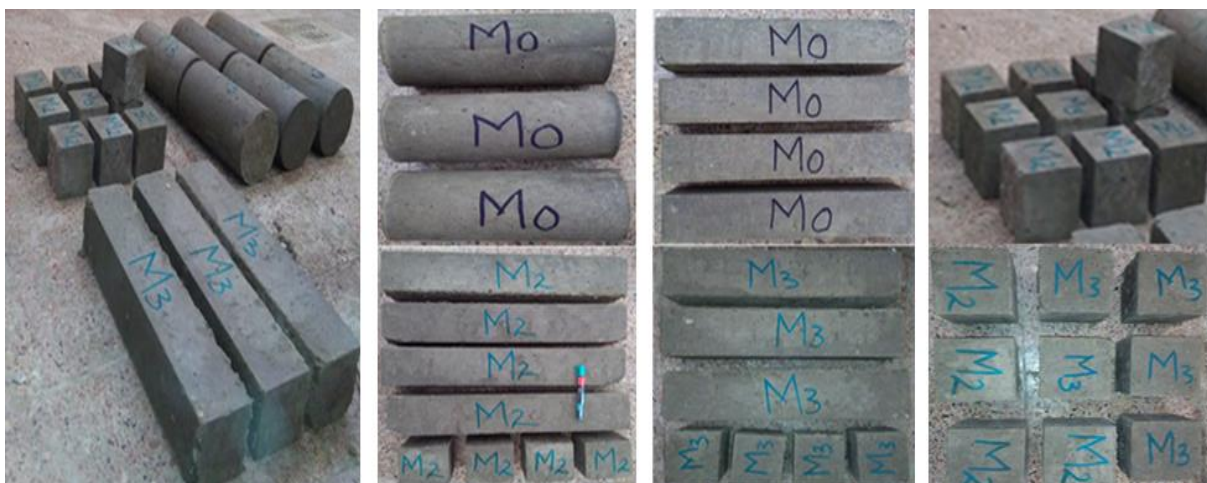
Figure 3.6: Cube, prism and cylindrical samples casted for testing
