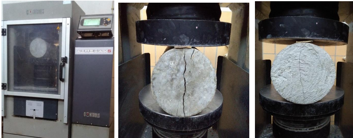
Photo: Split tensile strength testing machine and cylindrical specimens after loading
