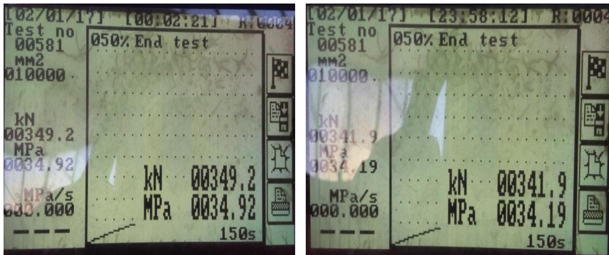
Photo: Compressive Strength test results for representative samples of mix M 1
