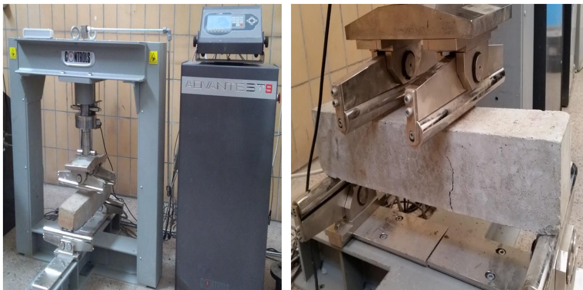
Photo: Flexural strength testing machine and beam under third-point loading
