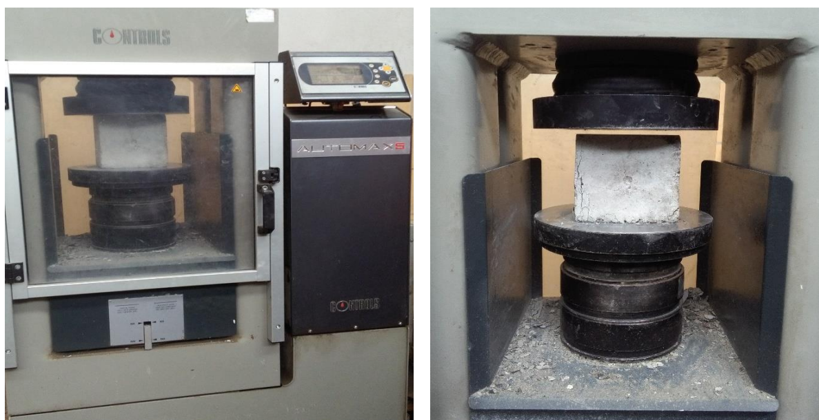
Photo: Compressive strength testing machine and cube samples under loading
