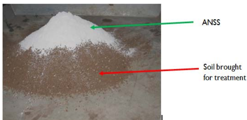
Figure 3.4: Mixing ANSS with soil for compaction test in the laboratory
