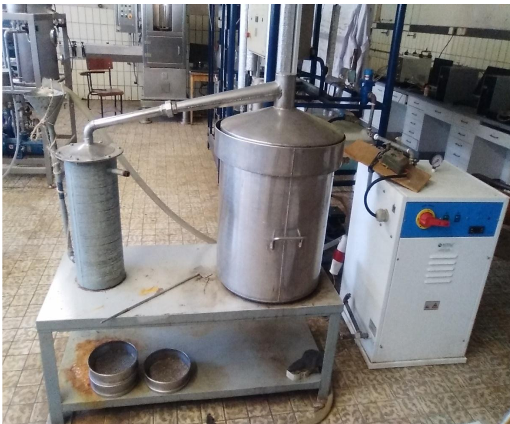
Figure 3.1 photograph of steam distillation equipment
