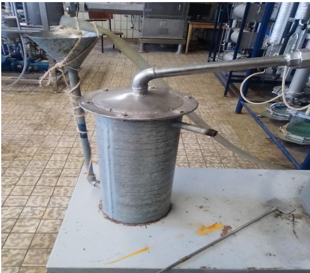
Figure 3.3 photograph of Shell and tube Condenser.
