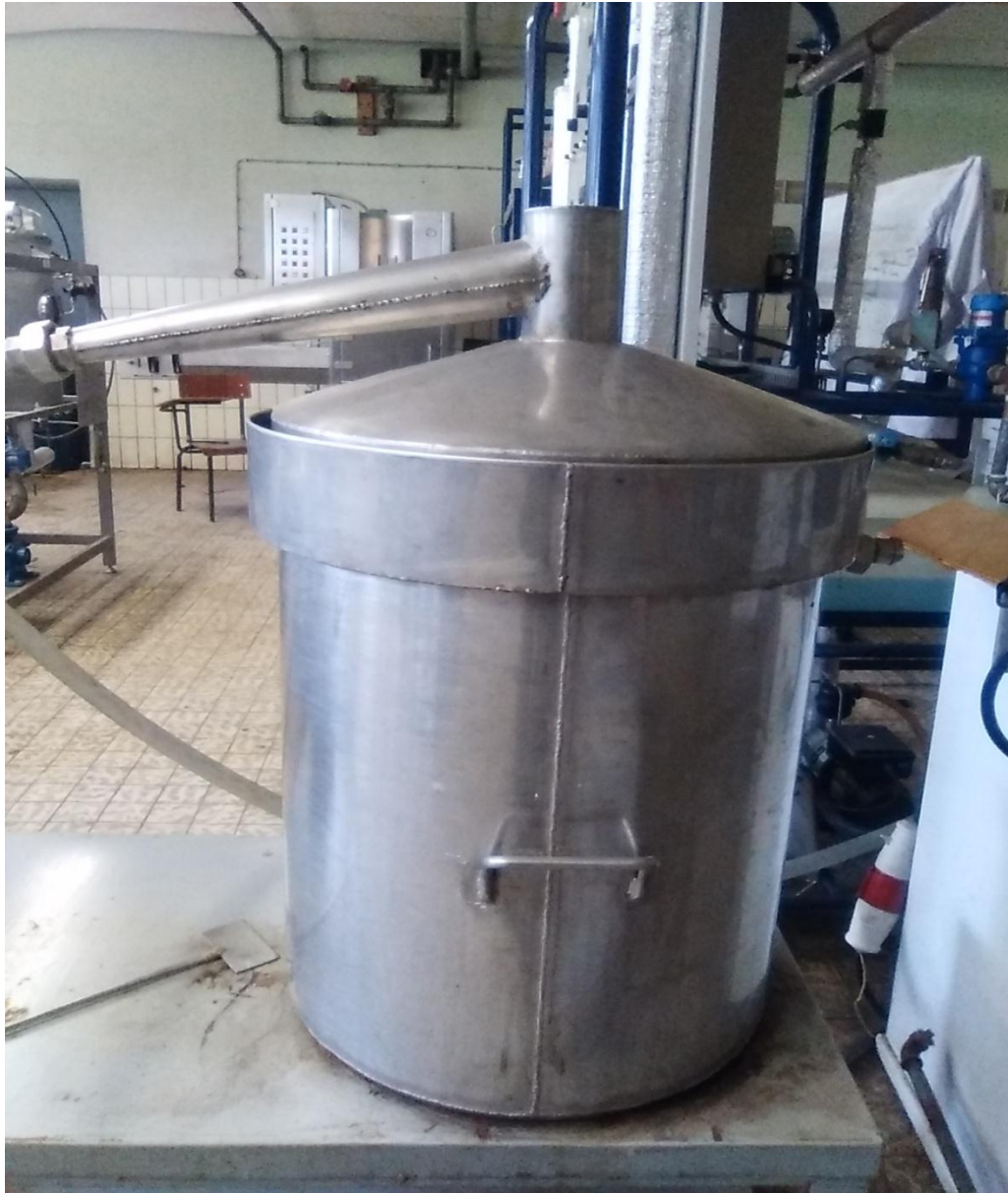
Figure 3.2 photograph of extraction chamber equipment
