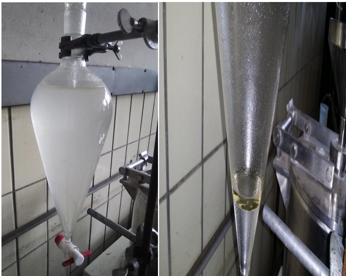
Figure C4: Gravity oil separator with pure essential oil and hydrosol
