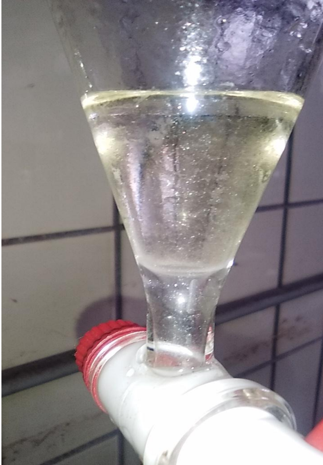
Figure C10. Pure rosemary essential oil inside gravity separator.
