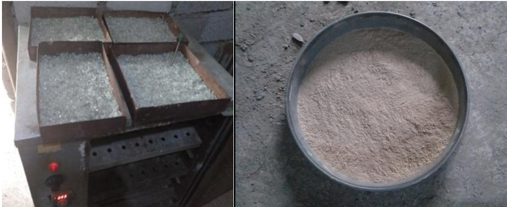
Fig. 3.1 Waste glass after oven dried (left) and waste glass after ground to powder (right).
