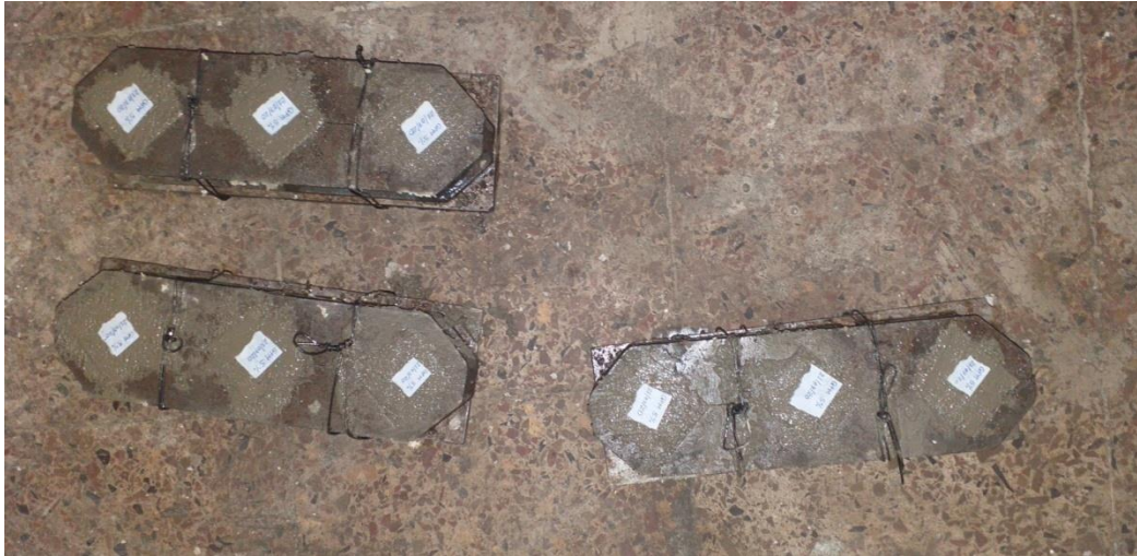
Photo 4. Mortar casted and troweled for compressive strength test.
