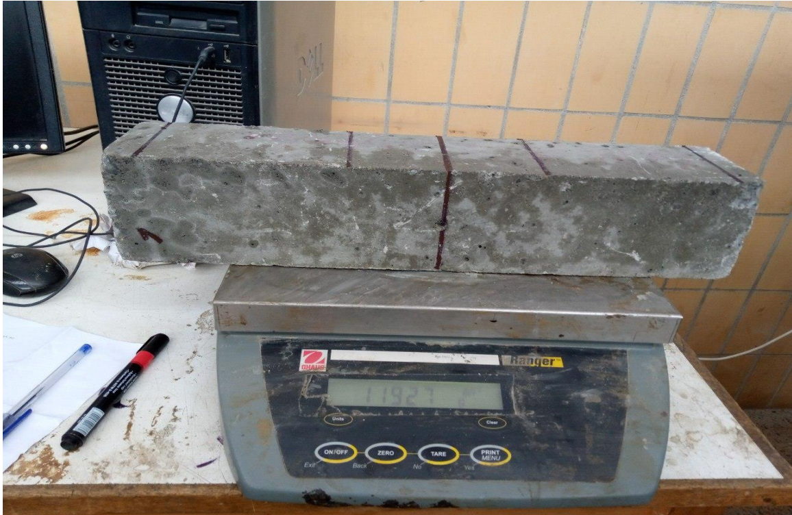
Photo 16. Concrete beam being weighed.
