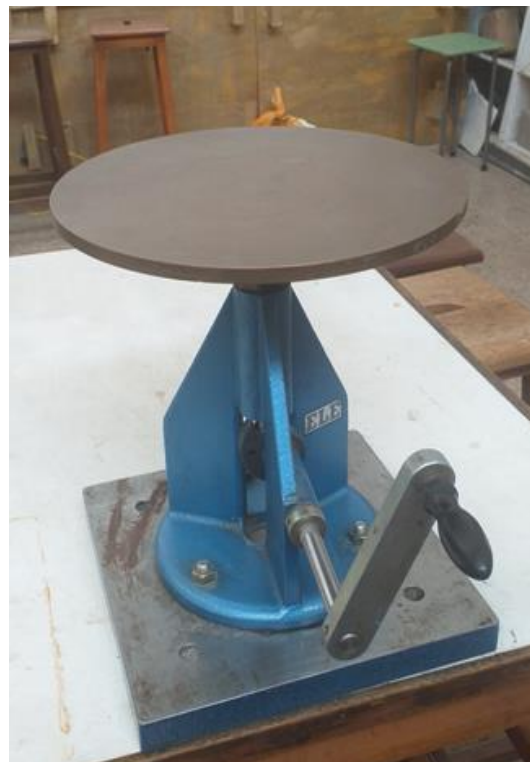
Photo 6. Flow table apparatus for mortar.
