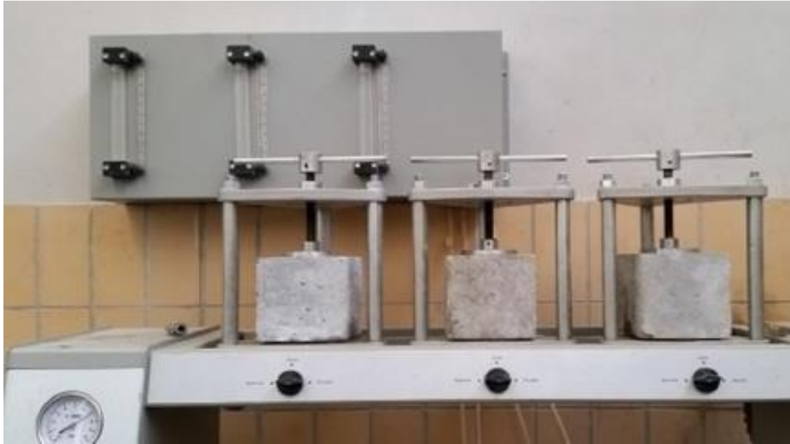
Photo 19. Concrete specimens assembled on water permeability testing apparatus.
