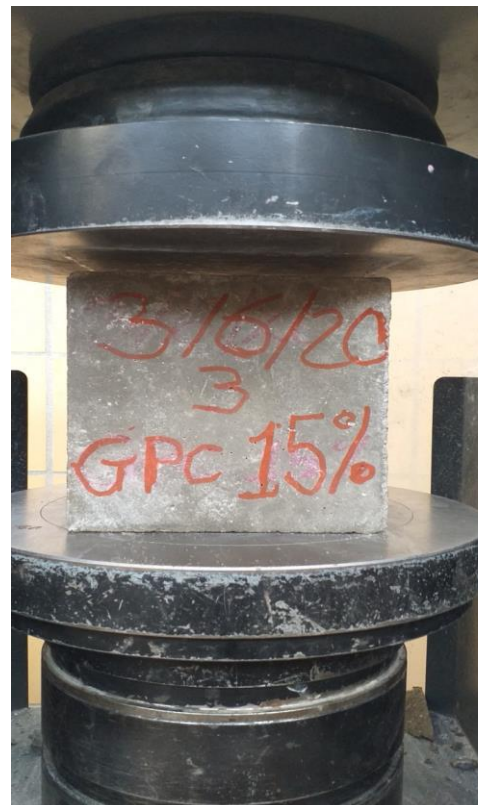
Photo 15. Concrete cube under compression test.
