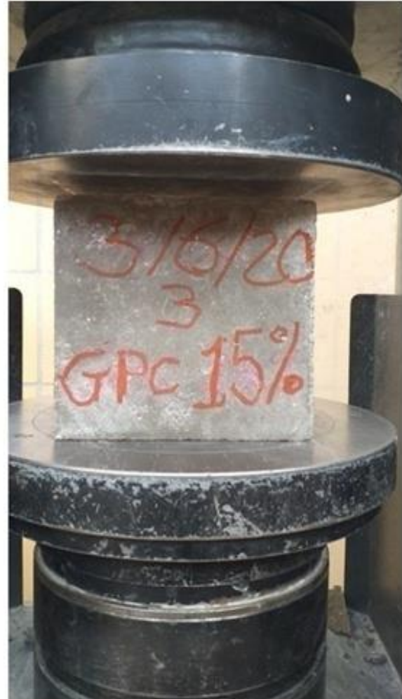
Fig. 5.13 Concrete specimen ready for compressive strength. Captured at AAiT material laboratory (2020).
