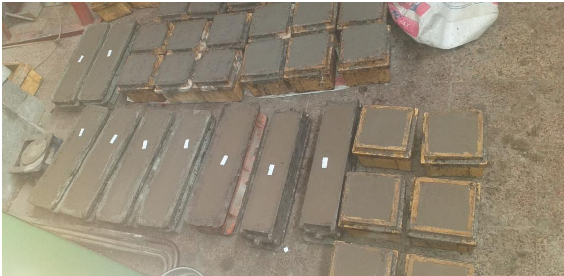
Photo 13. Concrete casted for compressive strength and flexural strength testing.
