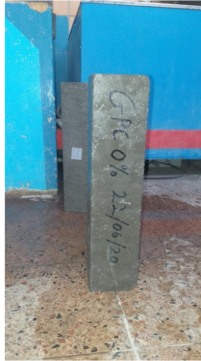
Photo 10. Concrete beam ready for flexural strength test.
