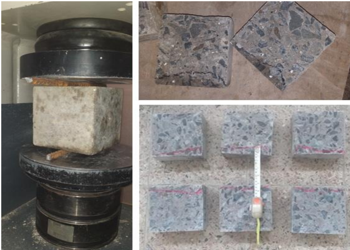
Photo 20. Splitting the permeability cube (left) and depth of water being measured (right).
