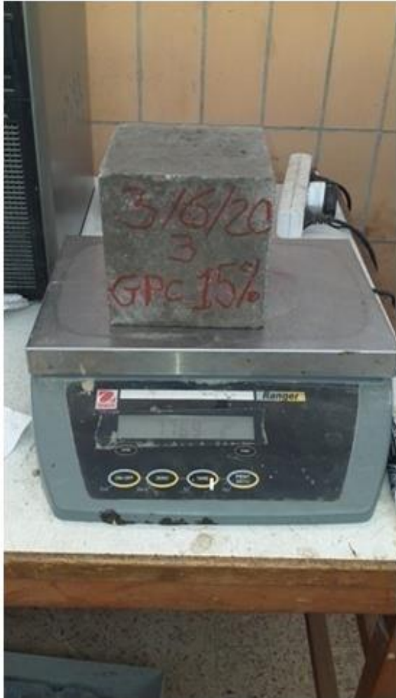
Fig. 5.12 Concrete specimen being weighed. Captured at AAiT material laboratory (2020).
