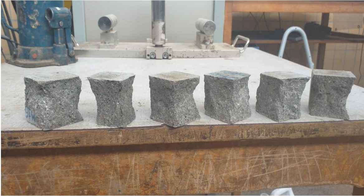
Photo 7. Mortar specimens after compressive strength test.
