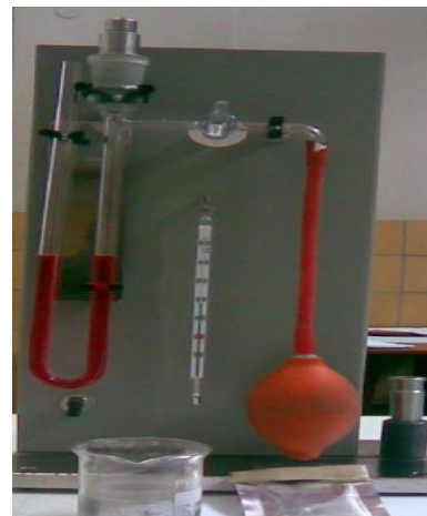
Photo 3. Blain air permeability apparatus.
