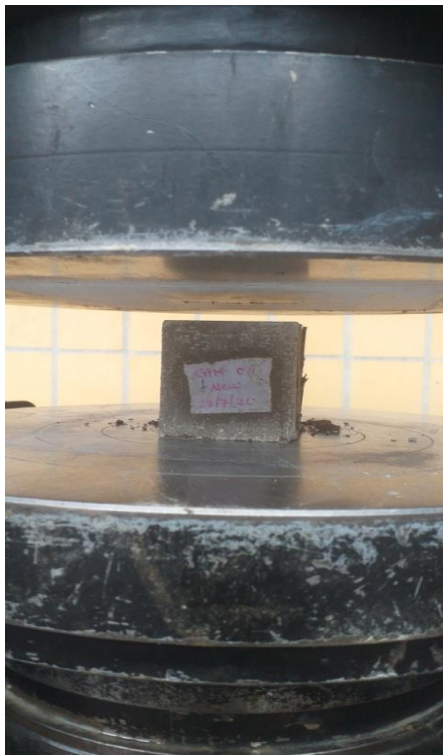
Photo 5. Mortar specimen under compression test.
