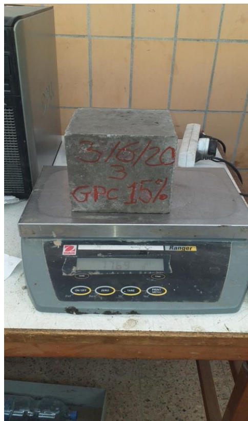
Photo 14. Concrete cube being weighed.
