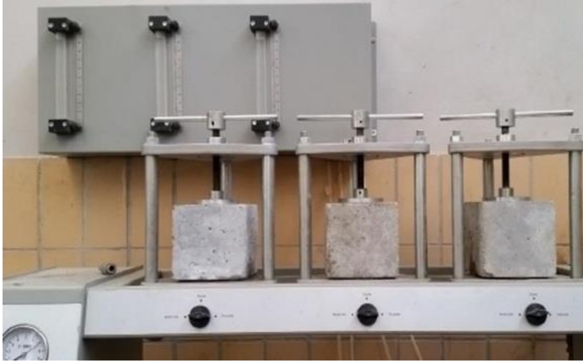
Fig. 5.17 Concrete specimens ready for water permeability test.
