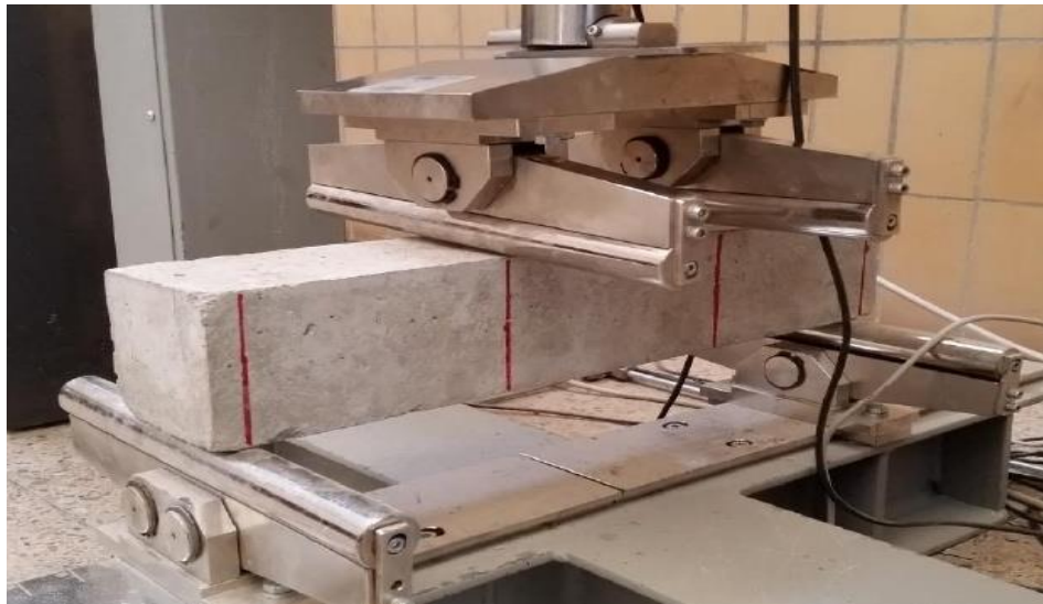
Fig. 4.1 Third point loading flexural strength test for Concrete beam.
