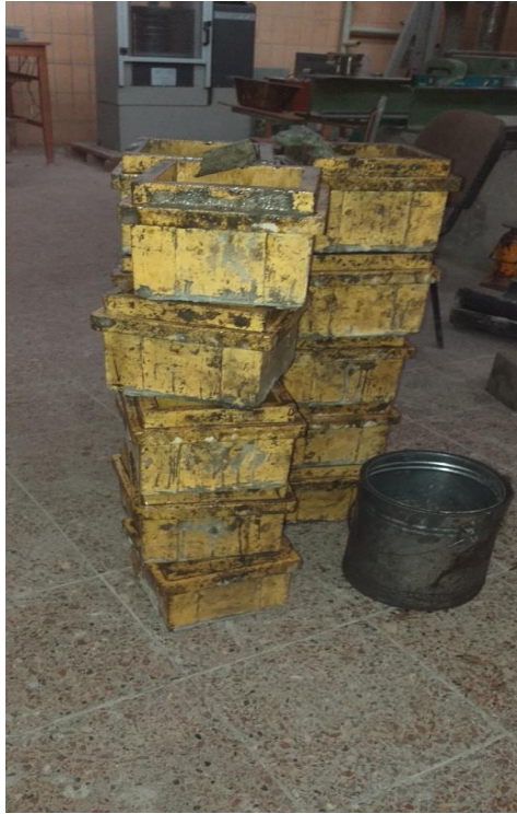
Photo 9. Oiled concrete molds.
