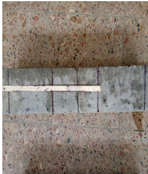
Photo 18. Concrete beam after flexural strength test
