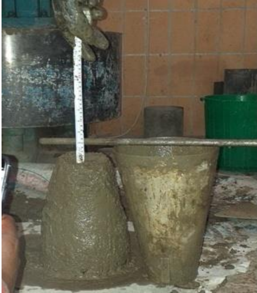
Fig. 5.9 Sample slump test of concrete.
