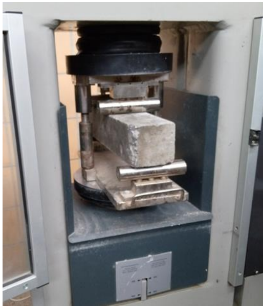
Photo 17. Concrete beam under flexural strength test
