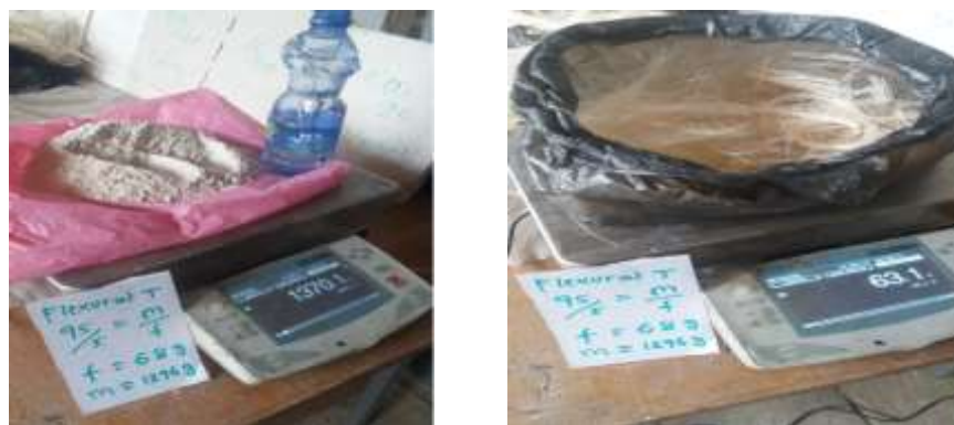
Figure 19 Gypsum and inset fiber weight for flexural sample
