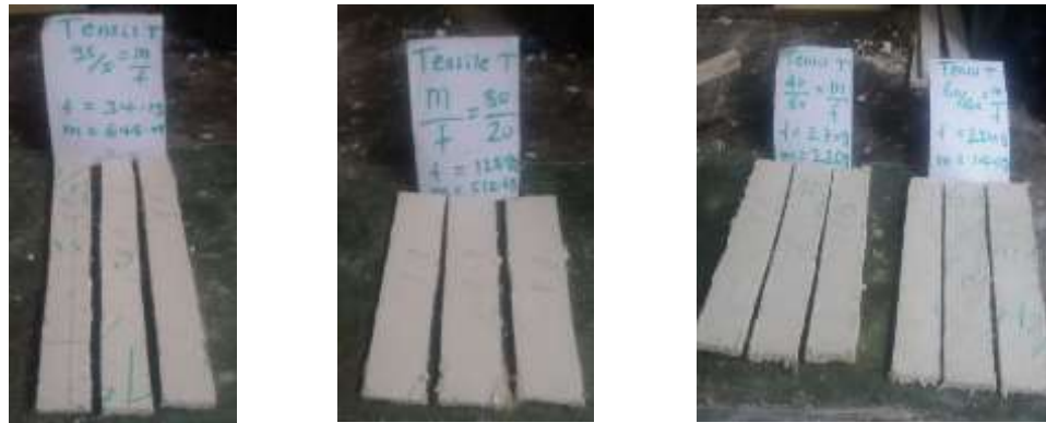
Figure 26 Specimens of composite material with Enset fibers and fibers in matrix
