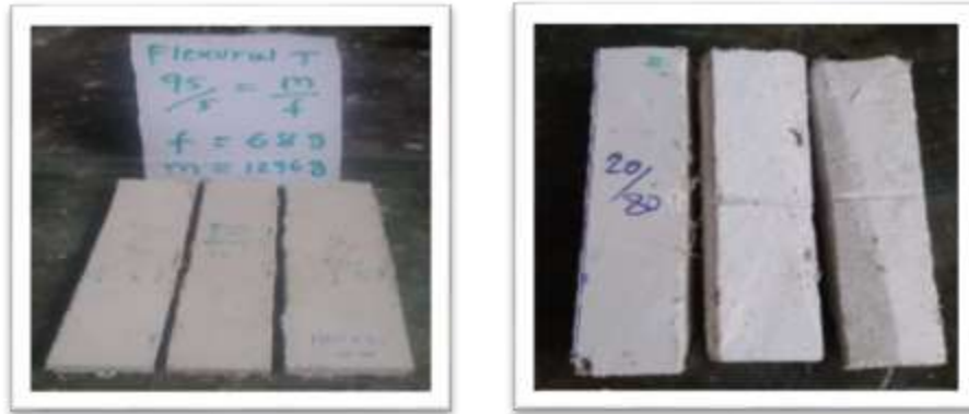
Figure 20 Prepared flexural sample to test Impact sample to test
