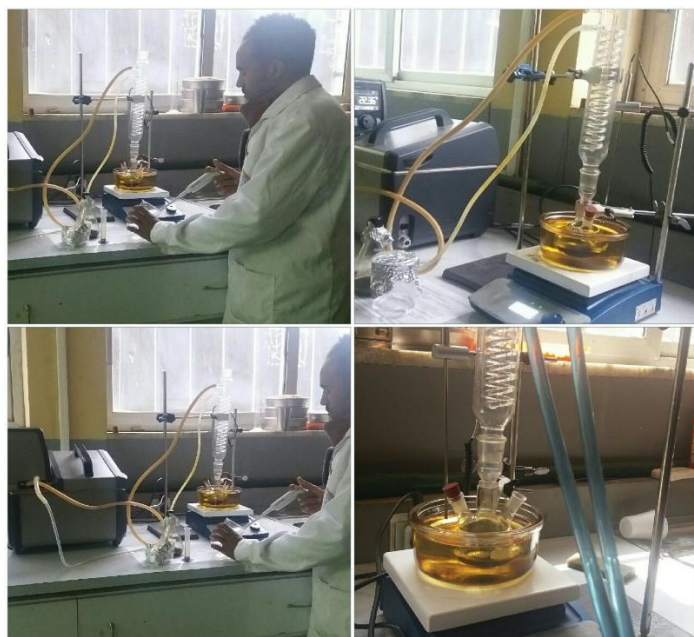
Figure 3-2 Experimental set-up for epoxidized vernonia oil production through epoxidation
