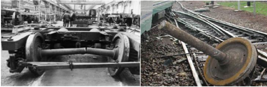
Figure 1-1 Broken Axles due to cyclic loading [5]
