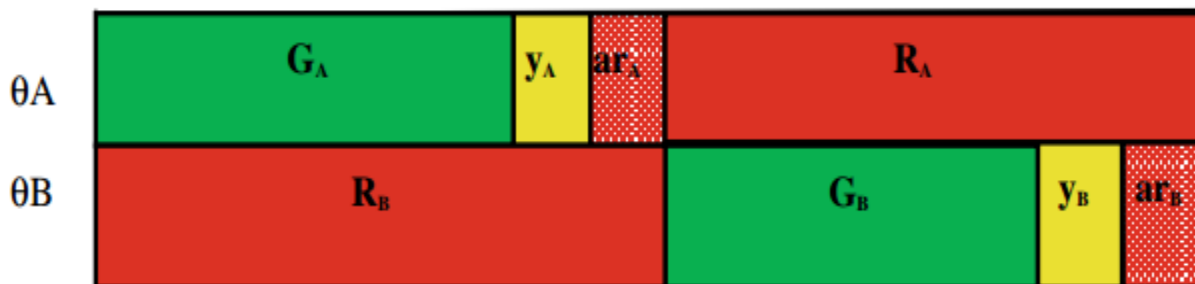
Figure 2.1 Relationships between Signal Intervals at Two Phase Signal
