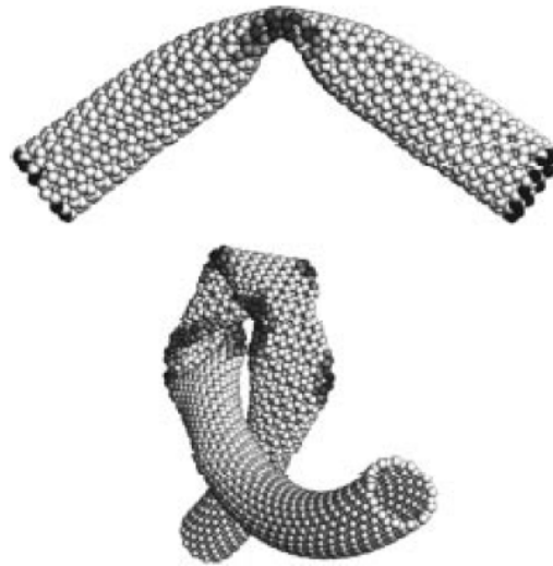
Figure 2.4: Simulation showing two possible ways, CNTs can deform or twist when they are loaded [24].
