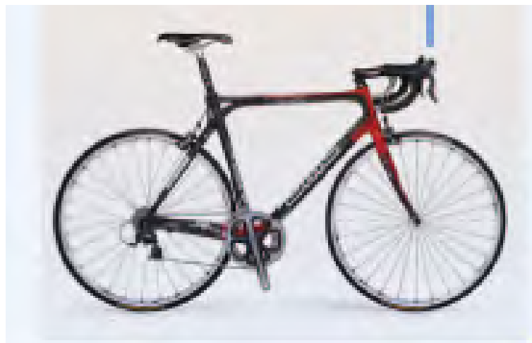
Figure 4.1: Winning Tour de France bicycle used carbon nanotube composite to make some parts of its body [41].
