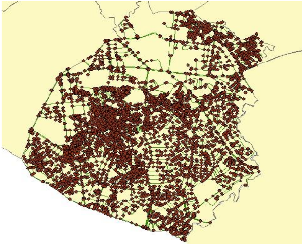
Figure 4.5 : Sample Road Junction Points
