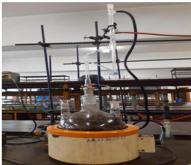
Figure 4: Hydro-distillation Clevenger apparatus set up used in essential oil extraction
