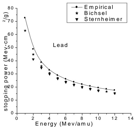
Fig.5.3 Stopping power of proton versus energy in Lead with others workers value
