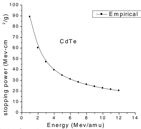
Fig.5.8 Stopping power of proton versus energy in CdTe
