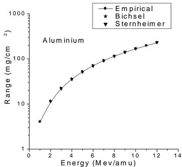
Fig.5.9 Empirical values for proton ranges versus energy in Aluminium with other workers value
