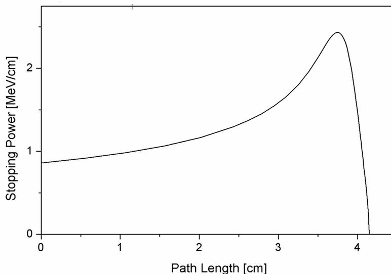
Fig 1.1 A diagram showing ionization loss versus distance from the sources for a beam of heavy charged particles in air at STP [3]
