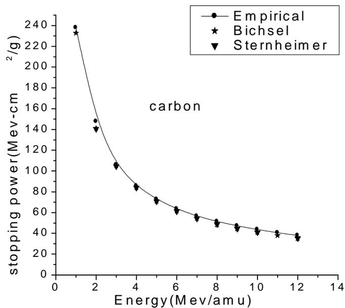
Fig.5.4 Stopping power of proton versus energy in carbon with others workers value
