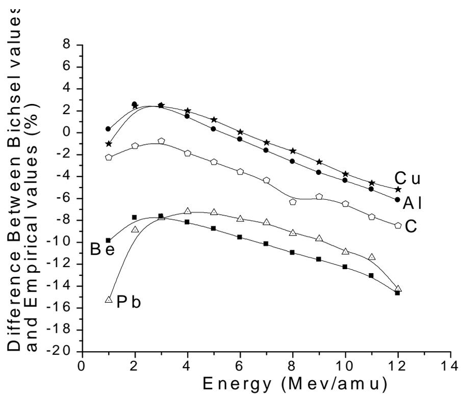
Fig 5.17 Percentage difference between Bichsel and empirical values of stopping power versus energy of protons
