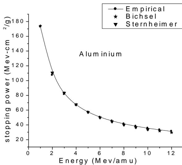
Fig.5.1 Stopping power of proton versus energy in Aluminium with other workers value
