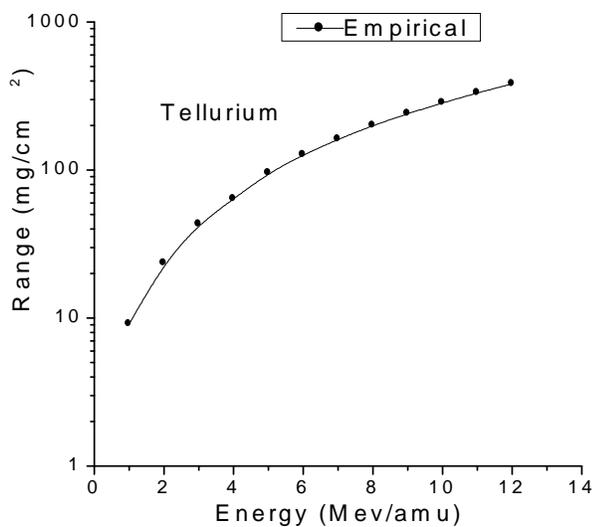
Fig.5.15 Empirical values for proton ranges versus energy in Tellurium
