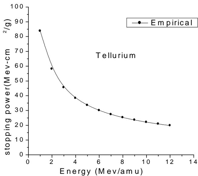
Fig.5.7 Stopping power of proton versus energy in Tellurium
