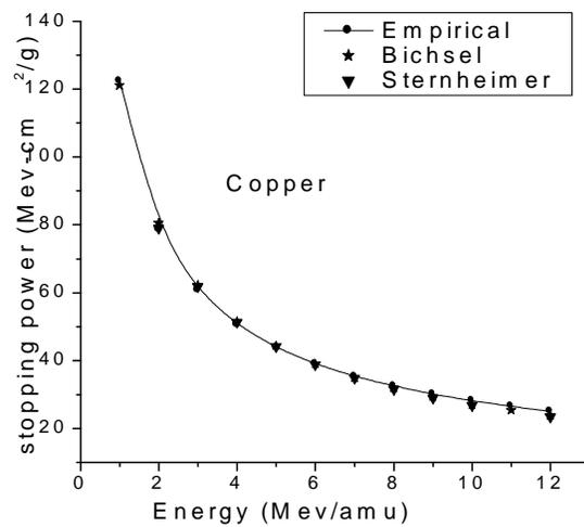
Fig.5.2 Stopping power of proton versus energy in Copper with other workers value
