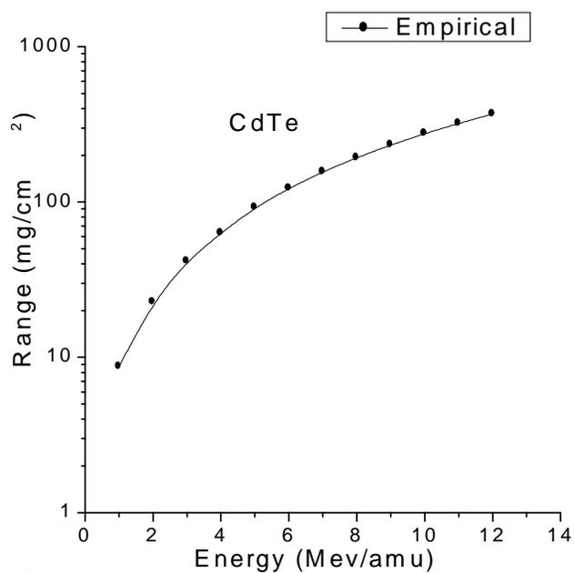
Fig.5.16 Empirical values for proton ranges versus energy in CdTe
