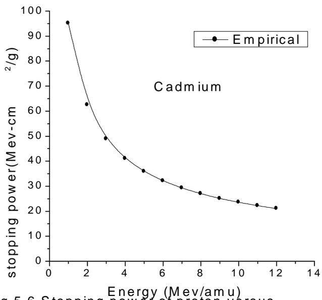
Fig.5.6 Stopping power of proton versus energy in Cadmium
