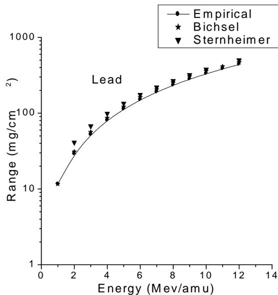
Fig.5.11 Empirical values for proton ranges versus energy in Lead with others workers value
