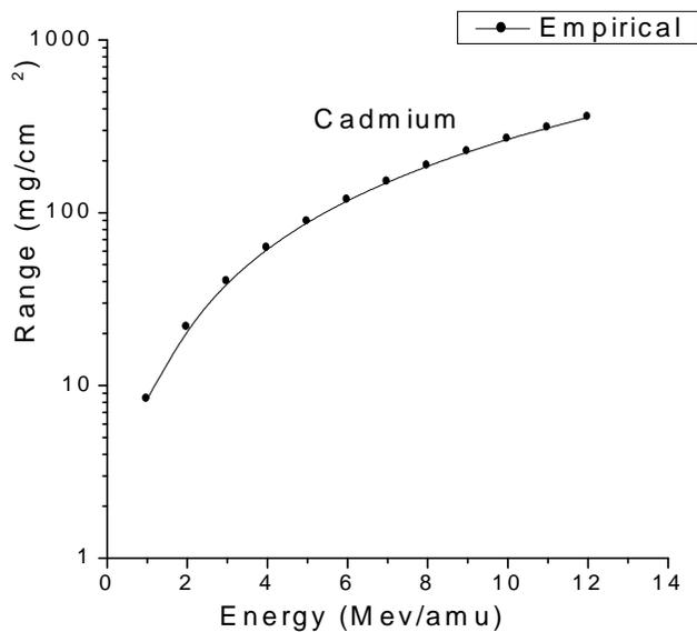
Fig.5.14 Empirical values for proton ranges versus energy in Cadmium
