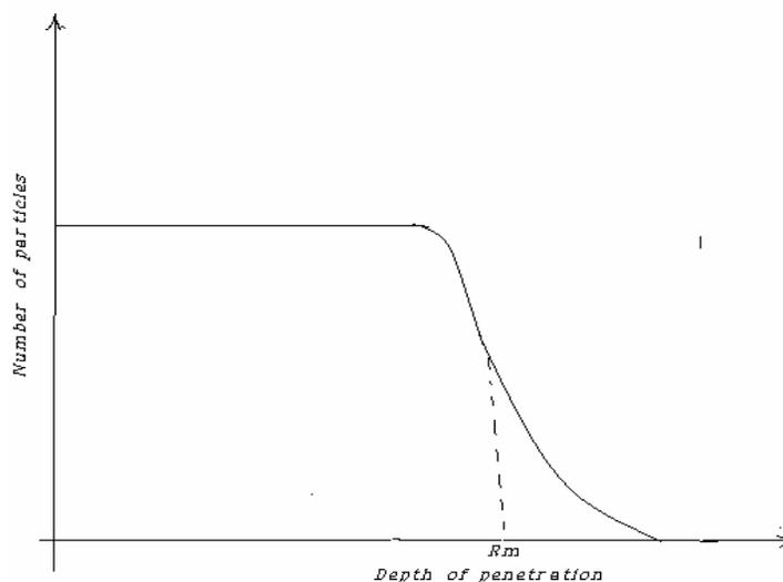
**Fig. (3.1) A diagram showing number of particles left versus depth in to an absorber.**
