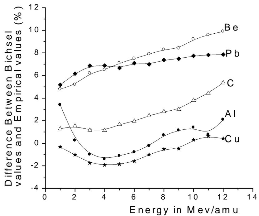
Fig.5.19 Percentage difference between Bichsel and empirical values of Range versus energy of proton.
