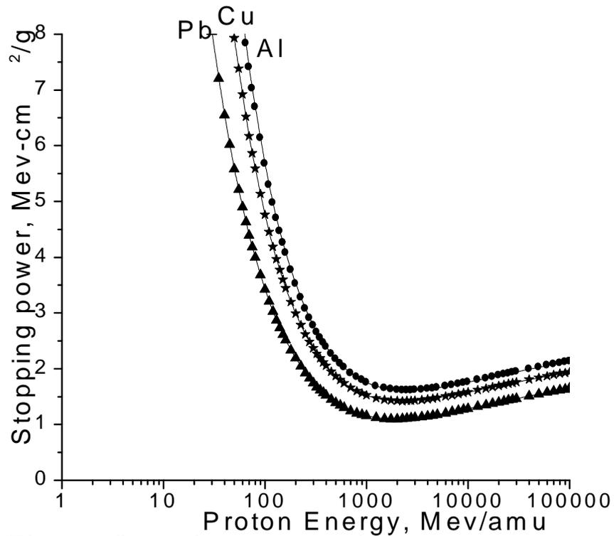
Fig.2.2 Stopping power of proton versus energy for Al,Cu,and Pb
