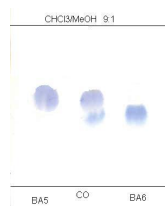
Fig. 8: Analytical thin layer chromatogram of BA5 and BA6
