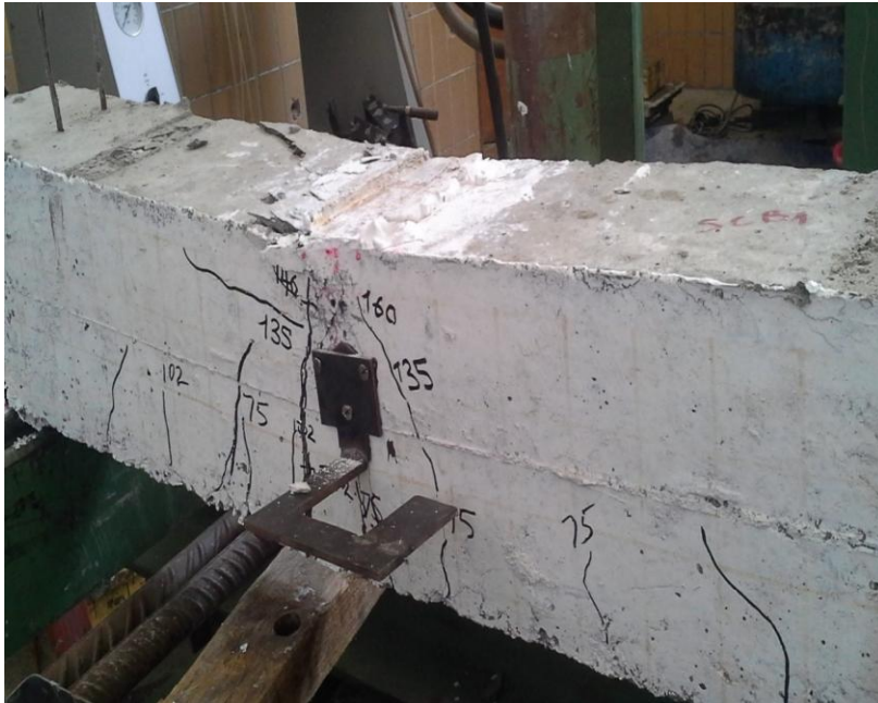
Figure A-3 Crack pattern and Load – deflection response (SCB1)
