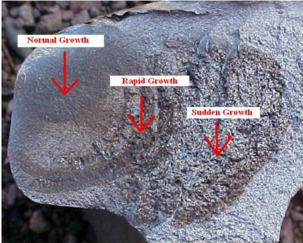
Figure 2-5 Detail Fracture Showing Normal, Rapid, and Sudden Growth Patterns [22].
