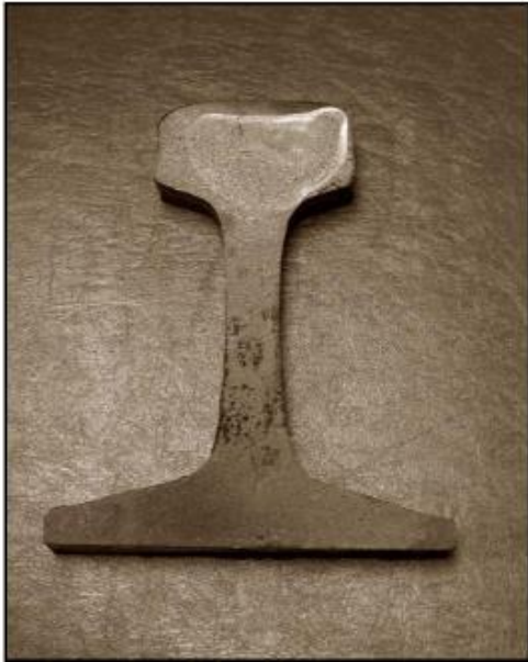
Defect shows extreme rapid growth pattern (rail end view)
