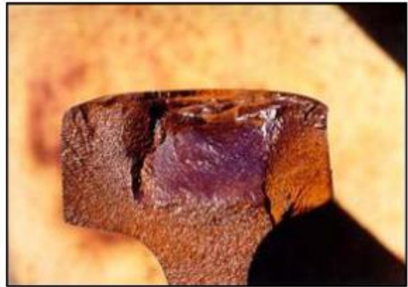
Engine Burn Fracture
