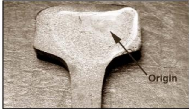
Defect shows extreme rapid growth pattern (rail end view)
