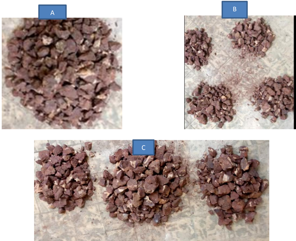
Figure 5: Cone and quartering method of sampling (A: cone shape, B: quartering: C: representative sample)
