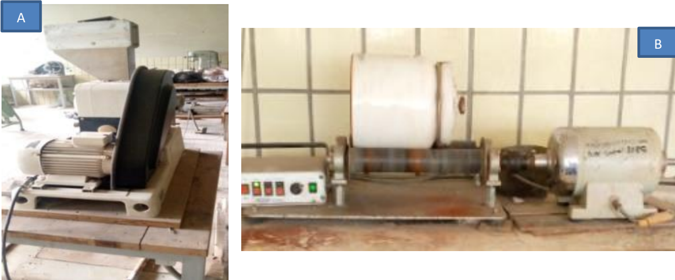
Figure 7: Laboratory Jaw crusher for primary size reduction (A) and ball mill for final size reduction (B)
