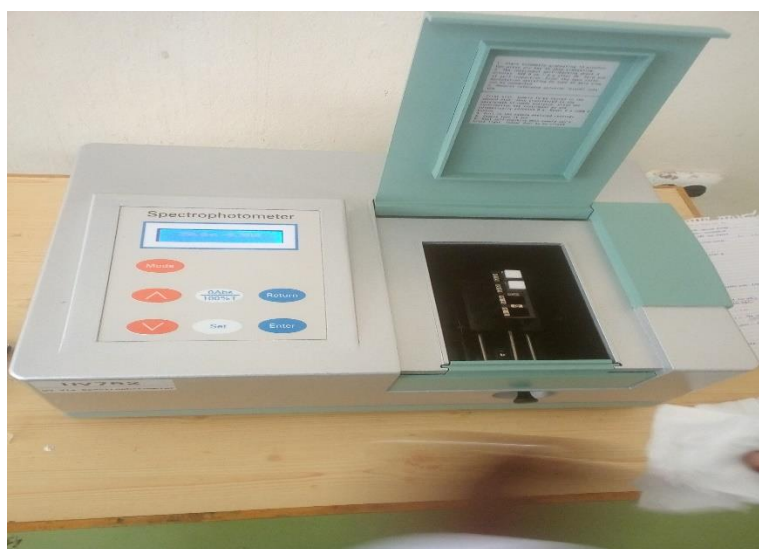
Figure 3-3: Acid Soluble Lignin Content Determination using Spectrophotometer
