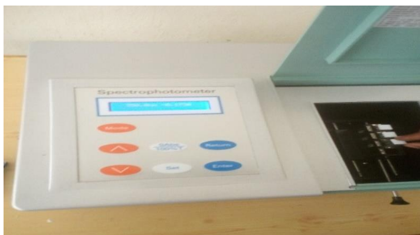
Figure 3-6: Kappa Number Determination using Spectrophotometer
