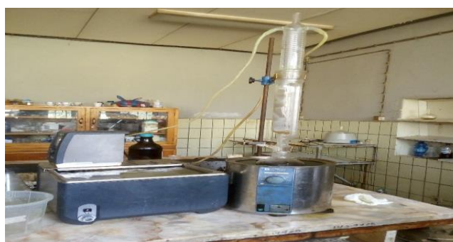
Figure 3-2: Removal of Extractive with Oil Bath Soxhlet Extraction
