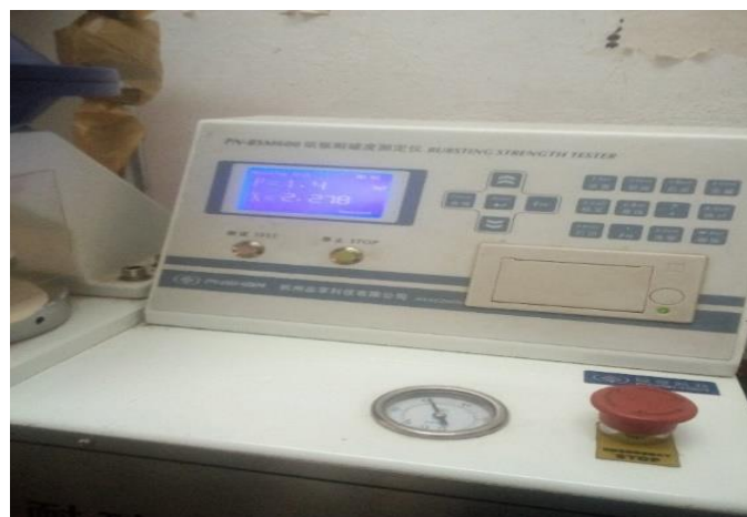
Figure 3-8: Bursting Tester Machine
