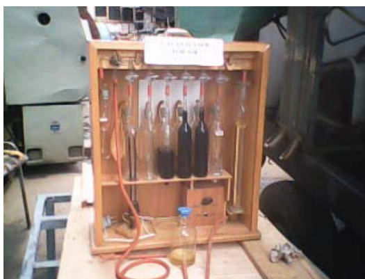
Figure 4-7 : - An Orsat gas analyzer
