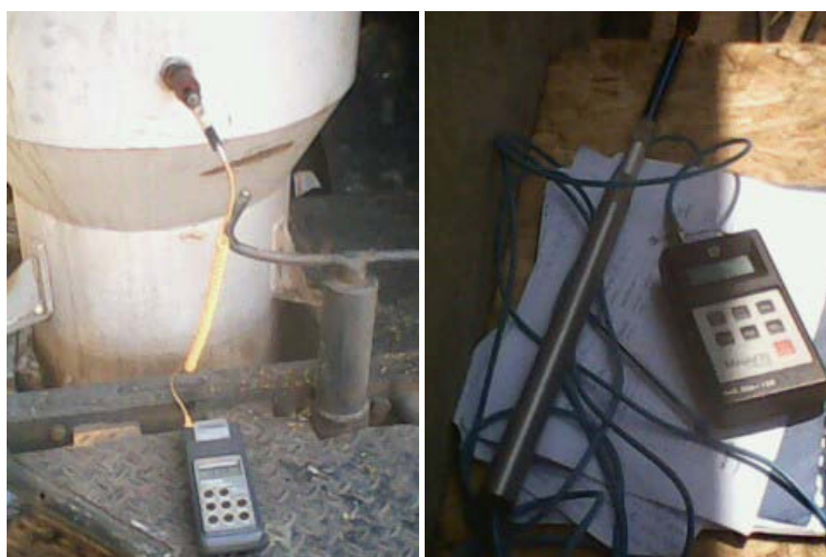
Figure 4-6 : - A K-type thermocouple (left) and vane type speed meter (right)
