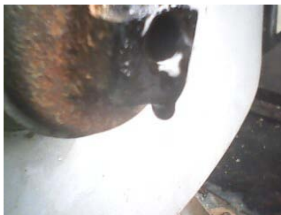
Figure 4-13 : - A highly viscous tar leaving through a tap hole near the pyrolysis zone
