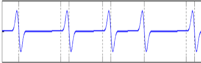
Fig.2.2 a PPM modulation scheme Fig2.2b BPSK modulation scheme
