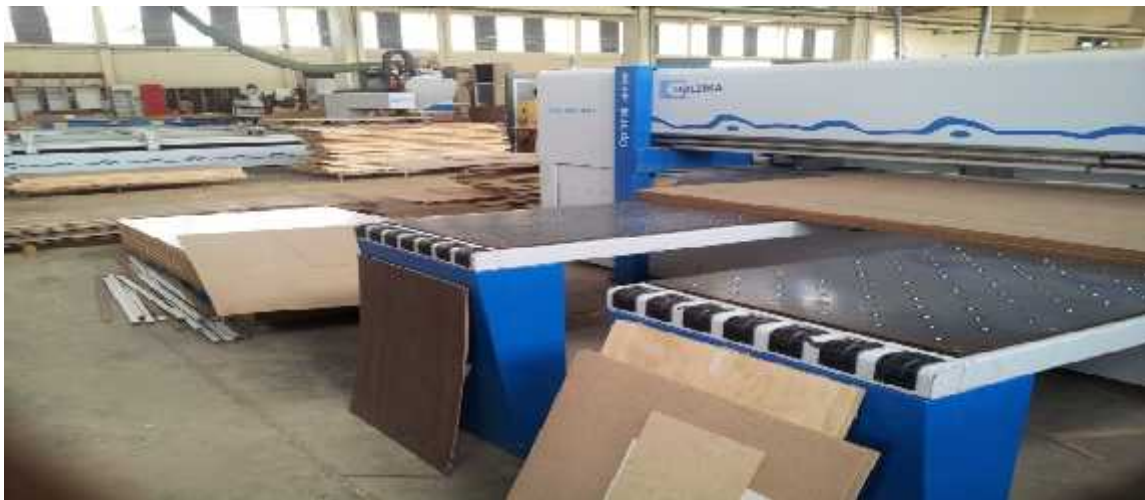
Fig.2.5: Panel cutting machine; source: photographed at the factory
